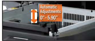
Automatic table height control from 0"-5.90.
