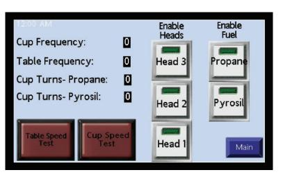
Enable Enable Fuel Heads 400 Cup Frequency: 400 Table Frequency: Head 3 Propane Cup Turns- Propane: 0 0 Cup Turns- Pyrosil: Head 2 Pyrosil able Speed Test Cup Speed Head 1 Main There are several operator options that can be selected. While both propane and Pyrosil are likely needed for your glassware, for stainless and powder-coat propane is likely all you will need for treatment.
