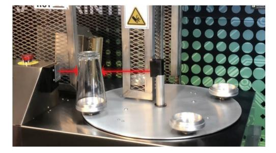
Once a cup has broken the line of sight the cup will stop in front of the flamehead,
