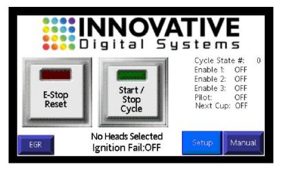
When the Pyrobond is turned on this is the home screen. To get started, select "Setup".
