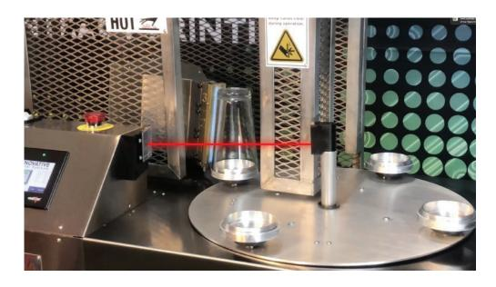
and based on options selected, the preset fuel and flameheads will fire, the cup will spin for each fuel source, once the cycle is complete, the table will turn.
