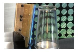
As you can see, we have 3 separate flameheads for each fuel source. This ensures that depending on the size of the cup, only the heads needed will flame.
