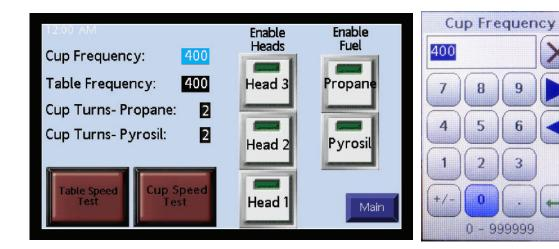
When you select a field, a numeric keypad will appear and allow you to make the necessary changes.
