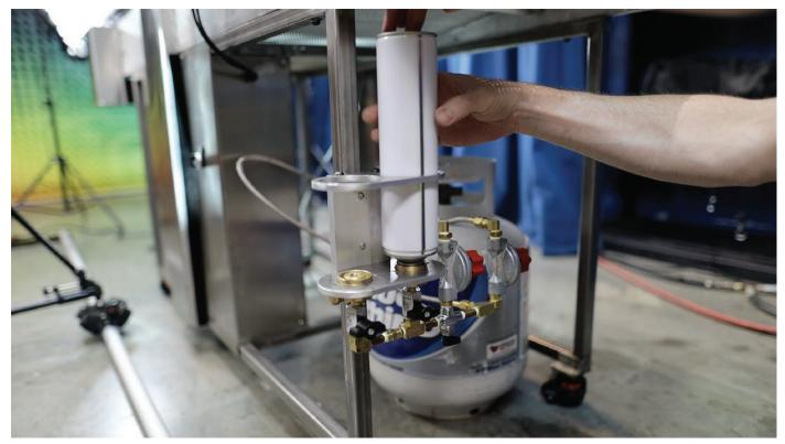
The Pyrosil connector is fixed to the Pyrobond GL. Simply remove cap from new canister and gently screw into place.
