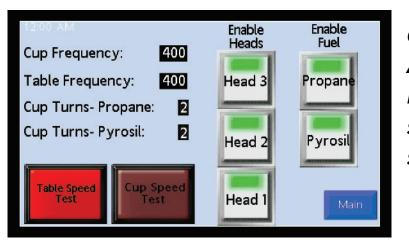
There are 2 test buttons to check the speed settings for the GL. Cup Frequency and Table Frequency. Before making any changes, select both test buttons to see how fast the table turns,
