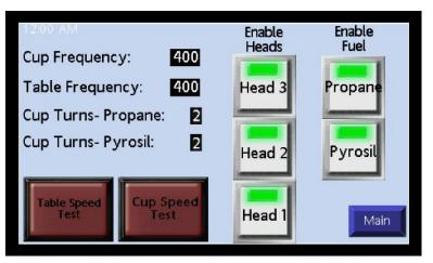
For this example, we will prepare the Pyrobond GL to treat glassware that will need 160° propane heat for pretreatment, and 2 turns of Pyrosil for maximum adhesion.
