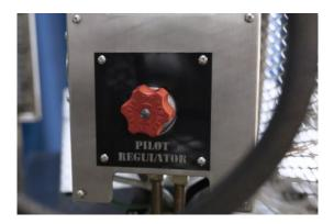
Once the fuel sources are installed, you need to open the valves for the pilot and the propane and Pyrosil. The propane has no gauge, but only needs be open enough to light the pilot.
