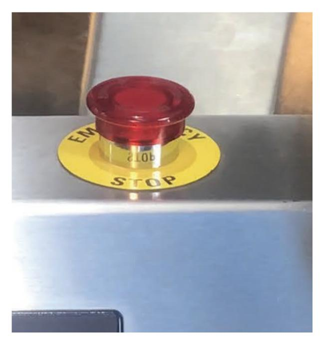
The emergency E-Stop is located in the front of the machine and right above the control panel for optimum access in case there is a need to stop the GL during a cycle.
