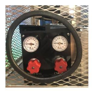
Make Sure the valves are opened and reading 10 PSI and that the pilot valve is opened as well.
