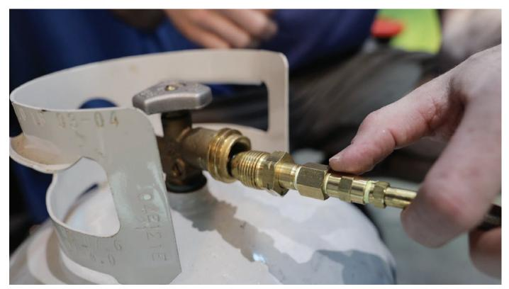
The propane connector is reversed threaded and is installed inside the propane tank valve. Turn counterclockwise in order to tighten connection.
