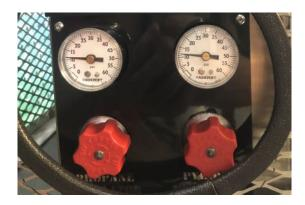
Found below the pilot value are the propane on left and the Pyrosil on right. While in use, both should be set to 10 PSI.
