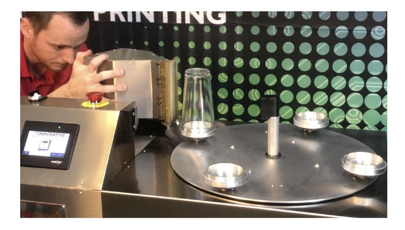
The Pyrobond GL is built on a sled, this makes adjusting the distance from flame to cup a breeze. There are 2 screws, and by using a 9/64" Allen key, loosening the aluminum clamp allows you to raise and lower flamehead. There are thumb screws to change the angle of flamehead, ideal for conical products.
