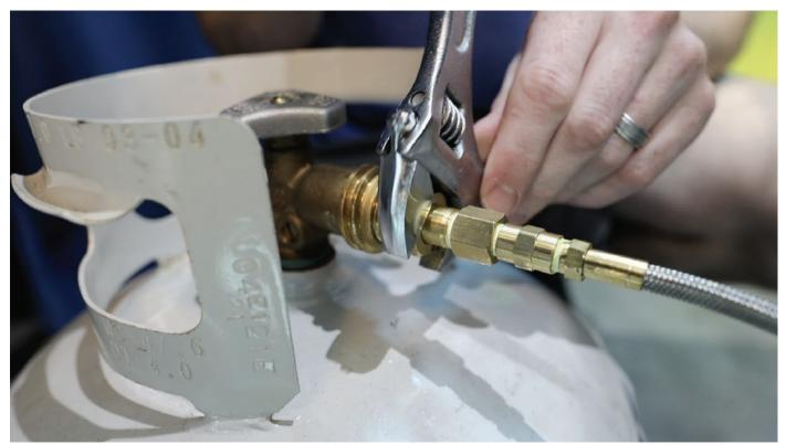
The propane connection should be a tight fit. Using a crescent wrench to complete install is recommended.
