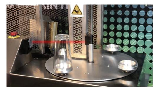
The laser sensor is designed to ensure the flamehead will only fire when a cup is detected, thus saving valuable resources.
