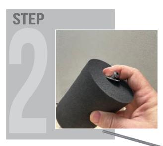
In this instance, we are installing the foam attachment designed for pint glasses. A 3/16" Allen Key will be needed to secure the foam attachment to the top of the included shaft.
