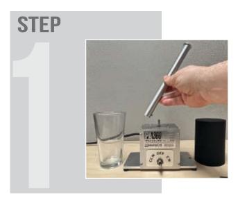
Select the appropriate fixture attachment to install on the PA 360 base unit. Need more tooling? IDS has a team of engineers that can custom design fixtures for your specific product needs.
