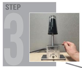
With a 3/32" Allen Key, tighten the set screw at the bottom of the shaft to secure it to the PA 360 base unit.
